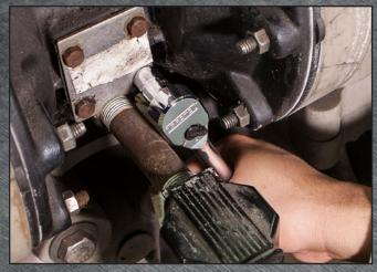
Patent pending sealed head design helps prevent debris from entering the ratcheting mechanism and helps to keep lubrication contained.
