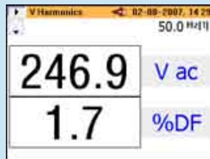
Harmonics measurements—view key harmonic factors such as distortion factor and total harmonic distortion, as well as individual harmonics up to the 30 th harmonic.
